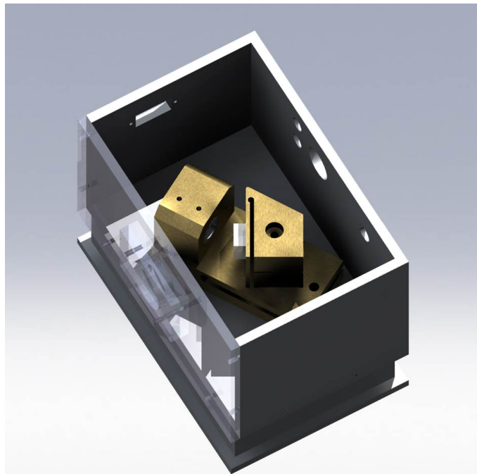
Figure B.1.: Render graphic of the home built external cavity diode laser. The cavity mechanics consist of a baseplate allowing for vertical adjustment of the grating with a fine threaded screw (Thorlabs; Ultra fine hex adjuster 3/16 100), a diode mount and a grating mount allowing for horizontal alignment of the grating via a fine threaded screw (Thorlabs; Ultra fine hex adjuster 3/16 100) and a piezo (Piezomechanik; PSt 150/4/5 bs). These parts are manufactured from nickel silver. The light is collimated by a collimation tube (Thorlabs; LT110P-B with standard lens (IR) and A110TM-A (423 nm)) and diffracted by a holographic grating (Thorlabs; visible holographic grating 1200/mm (IR) and 240/mm (423 nm)). Next to the collimation tube a temperature sensor (Conrad Elektronik; NTC 10k) is installed. A Peltier-element (Conrad Elektronik; Quick Cool 30 \times 30 \times 3.8 mm 8.6 V), positioned in between laser housing and cavity allows for temperature stabilization of the latter. The housing is made from anodized aluminium.
