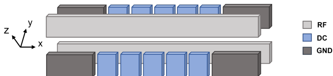
Figure 2.2: Schematic of a linear segmented Paul trap.
