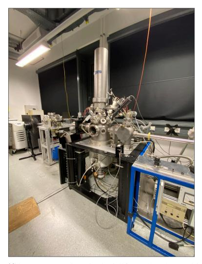
Figure 4 Photo of a time-of-flight mass spectrometry in a nuclear chemical laboratory (TOF-MS). Source: Christiane Schürkmann.
