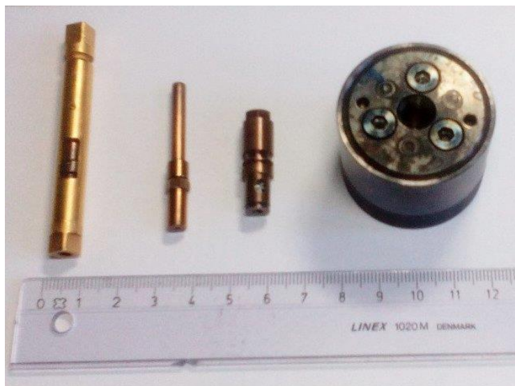
Fig. 2.4. High-pressure cells designed in Mainz (left to right: for magnetic studies up to 10 GPa, up to 1 GPa, up to 200 GPa loaded with H 2 S, and for Mössbauer studies up to 25 GPa). The photo is taken by the author, 2016.
