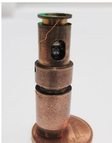
Fig. 4.1. High-pressure cell loaded with H 2 S. The photo is taken by the author, 2015.
