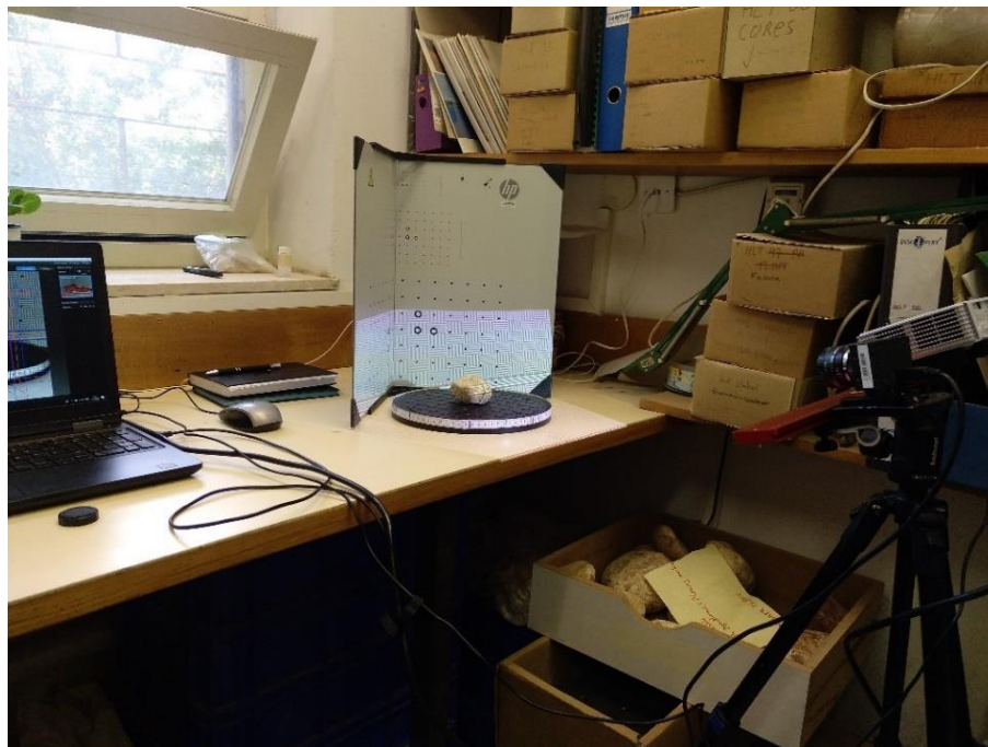
Figure 13: 3D scanning (HP 3D Structured Light Scanner Pro S3 DAVID) at the Hebrew University archaeological lab (Photo: Eduardo Paixão).
