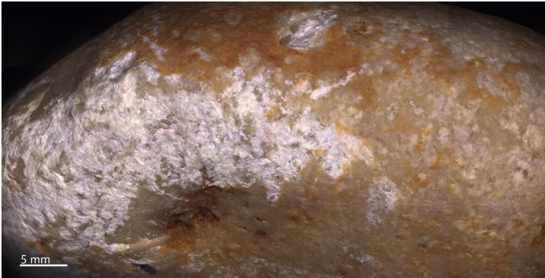
Figure 114: Smart zoom microscope image (34x): Sample 3-3 (50 impacts on flint).
