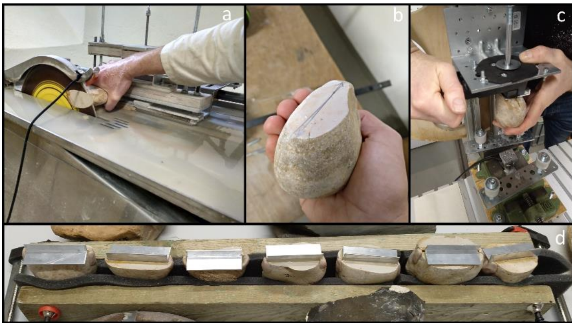
Figure 18: Sample preparation for mechanized experiments: a) cutting a surface opposite to the active area b) marks to cut the groove c) sample installation in the sample holder d) fixing the metallic adaptor to the tools (Photos: Eduardo Paixão).
