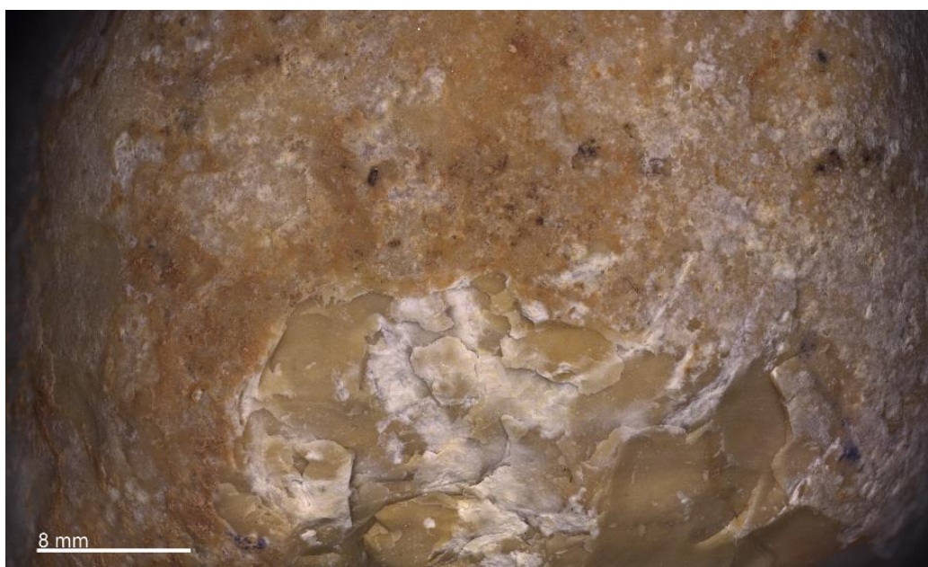
Figure 113: Smart zoom microscope image (34x): Sample 3-12 (50 impacts on flint).
