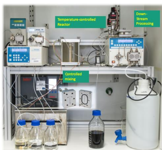
Fig. 1 Photograph of the micromixer platform used for synthesis of single core iron-oxide MNP.
