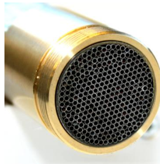
Figure 10. Laminar Flow Element with a set of 1 mm cannulas cut by wire EDM.
