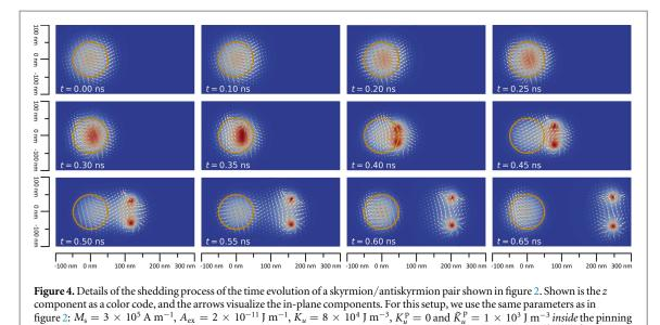
area which has a radius of 50 nm, Gilbert damping of  $\alpha = 0.05$ , and  $\beta = 0$ . The applied current density is 5  $\times 10^{12}$  A m<sup>-2</sup>.
