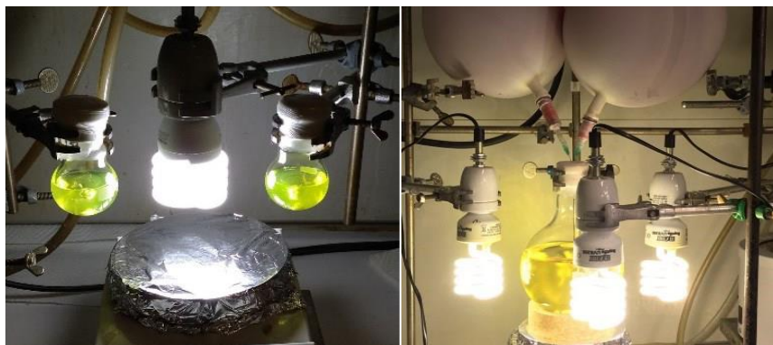
Figure 31. Set-up of preparative photoredox reactions with a 25 W UV/Vis-CFL (left) and with a 23 W Vis-CFL household lamp as a multigram scale approach (right).
