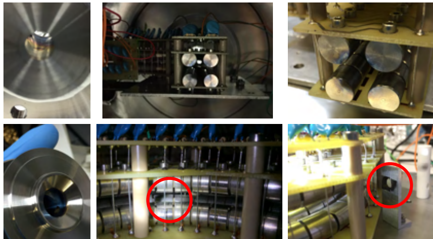
Figure 4.15.: Visible contaminations of the flow channel (left) and the RFQ rods (middle and right) after the beam time campaign. The jet cell CF40 window for the anticollinear laser beams was coated as well, but no picture taken.
