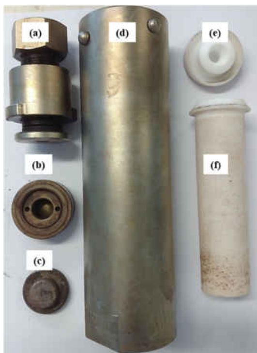
Figure 9. Photograph of a typical Morey-type autoclave, which was used in this work, with its single components: (a) stainless steel lid with plunger, (b) seal and bursting disc, (c) cylindrical pin, (d) stainless steel case, (e) Teflon ® -lid and (f) Teflon ® -lined vessel.
