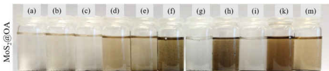
Figure 112. Solubility experiments of the MoS 2 @OA nanosheets in various solvents: (a) ethanol, (b) 2-propanol, (c) acetone, (d) ethyl acetate, (e) hexane, (f) benzyl alcohol, (g) water, (h) chloroform, (i) acetonitrile, (k) toluene and (m) DMF.
