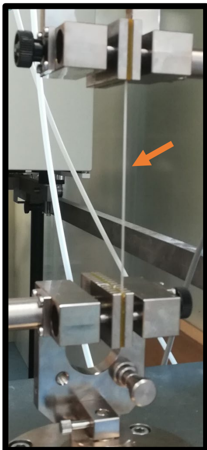
Figure S 28: Picture of the strained film of TPE-1 (left). Picture of the strained (torn) and the unstrained film of TPE-1 (right).
