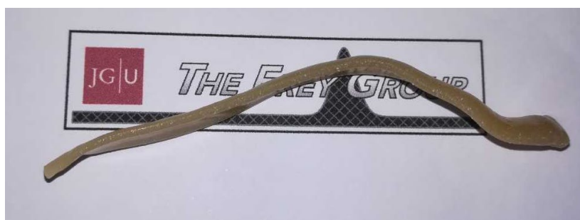
Figure S 22: Extrudate filament at 140 °C with 140 min -1 extrusion speed with 4 wt% of asparagine.
