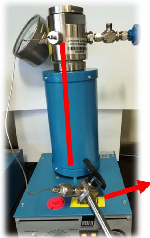
Figure S 19: Image of the autoclave used for the kinetic studies.
