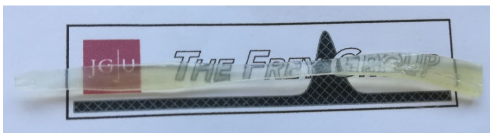
Figure S 20: Extrudate filament at 140 °C with 140 min -1 extrusion speed with 500 ppm Irganox®.
