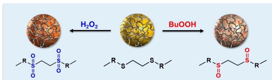
Figure 2.1.8. Selective oxidation of polythioethers (S(II)) with tert-butyl hydroperoxide to the partially oxidized polysulfoxides (S(IV)), and with hydrogen peroxide to the fully oxidized polysulfones (S(VI)).
