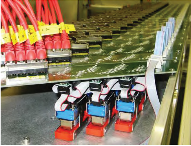
Figure 2.52.: Photograph of the assembled read-out and front-end electronics for the first plane of the fibre detector, that is mounted on top of the vacuum chamber flange which is shown in Fig. 2.48.
