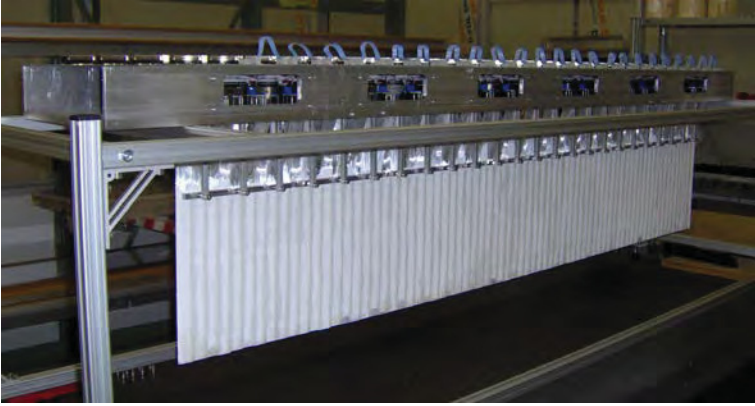
Figure 2.48.: Photograph of the assembled first plane of the fibre detector taken in a clean room during assembly in 2008–9. The plane is composed of 9 216 fibres in 72 bundles and attached to the vacuum chamber flange through leak-proof fibre connectors.
