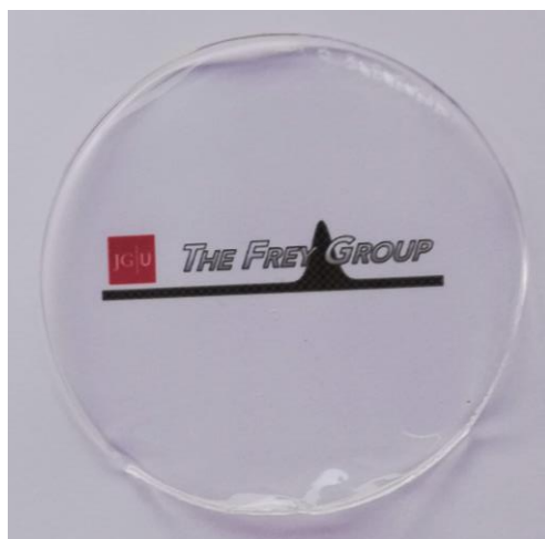
Figure S22. Exemplary transparent film of PS_{0.25}\text{-}co\text{-}P(\text{Far}_{0.5}\text{-}b\text{-}S_{0.25}) , cast by solvent evaporation of a chloroform solution ( c = 20 \text{ wt}\% ).
