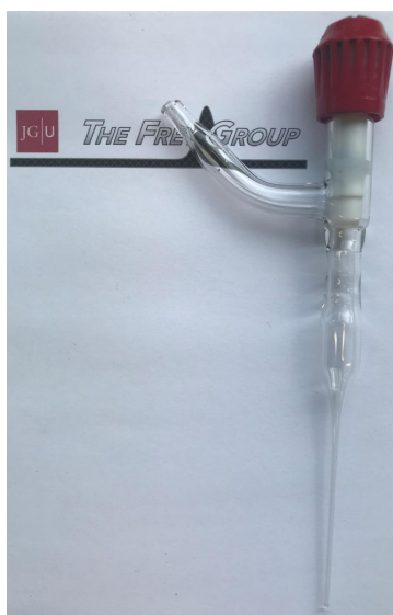
Figure S1. Special designed Schlenk-ampule for in situ NMR kinetic measurement of polymerization of PO and D 3 in DMC catalysis.
