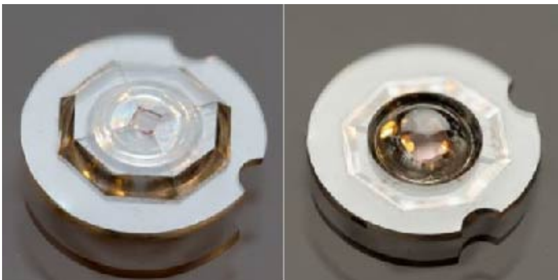
FIGURE 7.5: Constructed diamond optical assembly, the left side depicts the front side of the optical assembly (before HR coating) and the right side the back of the assembly.
