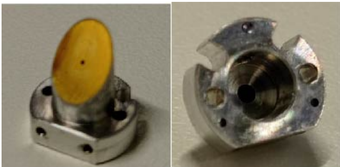
FIGURE 7.10: Photograph of the MPD00M9-M01, Thorlabs parabolic mirror after processing from the JGU workshop.
