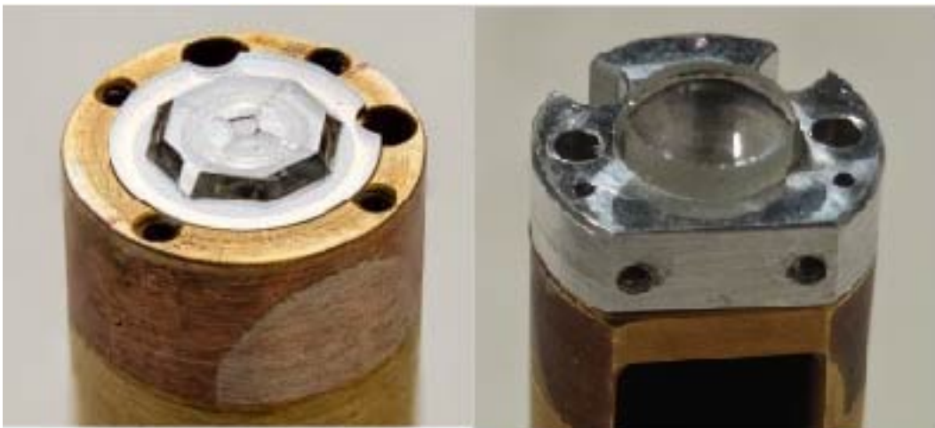
FIGURE 7.12: Picture of the sensor with the three major pieces attached to one another. The left side shows the front side of the sensor and the right side shows the back side of the sensor.
