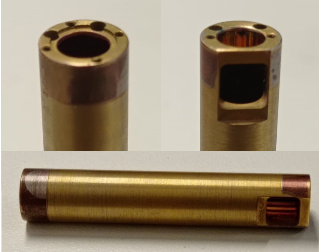
FIGURE 7.8: Copper pipe after electroplating as seen from different points of view.
