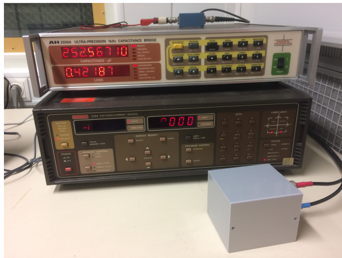
(a) Closed setup with capacitance bridge and DC voltage source in the background.
