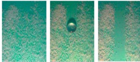
Figure 2.3.1: Self-cleaning surfaces, a 20 \mu\text{L} water drop deposited carries away silica particles (particle size ranges from 0.2 \mu\text{m} to 0.5 \mu\text{m} ) deposited onto a liquid-infused surface lubricated with silicone oil inclined by 20°. Reproduced with permission from Lafuma and Quéré, 2011, EPL , 96, 56001. Copyright © 2011 IOP Publishing, all rights reserved.
