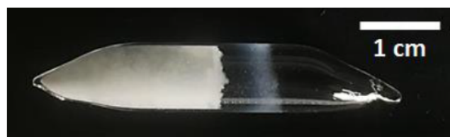
FIGURE 6.11: \text{MgCl}_2 sample prepared for irradiation at the Institute Laue-Langevin. The \text{MgCl}_2 sample is filled into a quartz tube under helium atmosphere.
