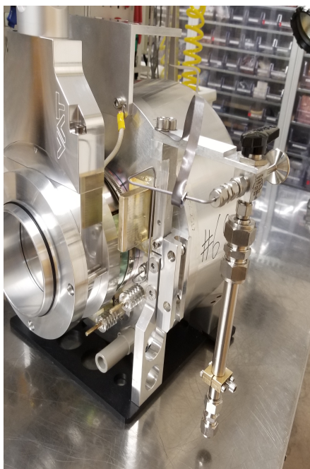
FIGURE 5.14: KENIS ion source with external caesium reservoir mounted on the target.
