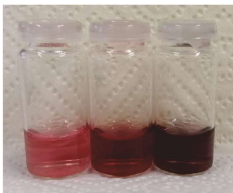
Figure 28: Gold nanoparticles and their optical colour perception with increasing diameter (from left to right) of the nanoparticles.
