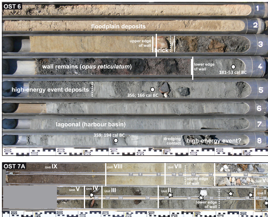
Fig. 6 Photographies of vibracores OST 6 and OST 7A. core OST 6 penetrated an opus reticulatum wall that originally separated vaulted chambers of the navalia-temple complex. Radiocarbon ages are given according to Hadler et al. (2015). Core 7A shows the sedimentary infill of chamber W4. Hexagons mark position of radiocarbon samples retrieved from core OST 6 with calibrated ages ( 2\sigma ) already published by
