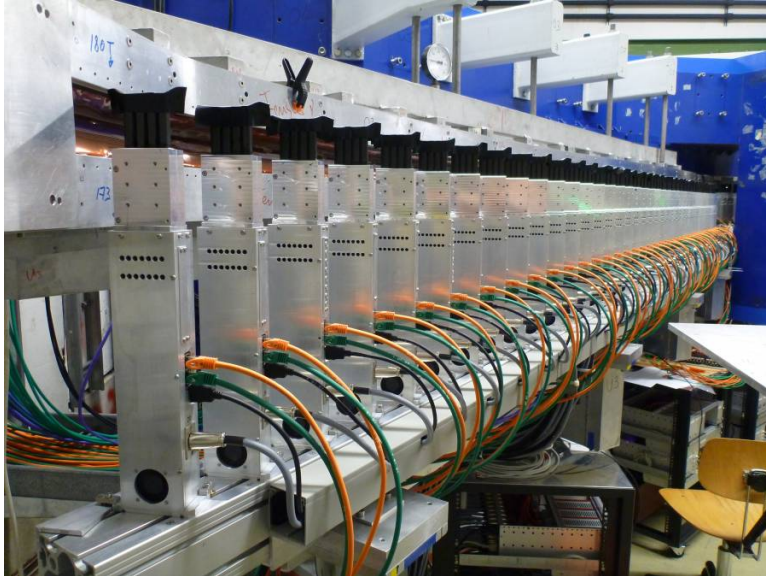
Figure 4.10: Picture of the new modular detector of the tagging spectrometer [104].
