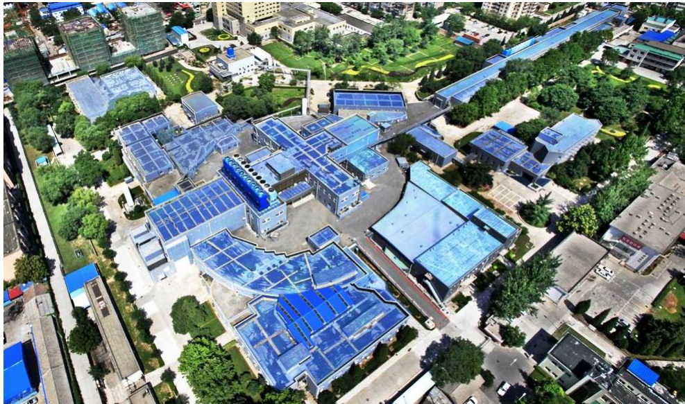
Fig. 3.1: View on the BEPCII facility center with the collider ring in the middle of the picture and the linac in the upper right part, located at the IHEP in Beijing. The BESIII detector is situated at 8 o'clock on the ring. (Original image from http://www.ihep.ac.cn )
