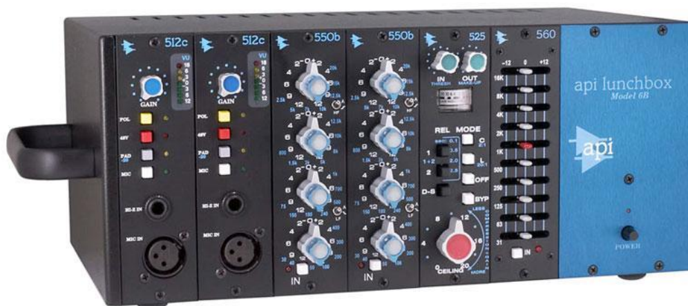
Figure 18 The API lunchbox, a rack for mounting 500-format processors.
