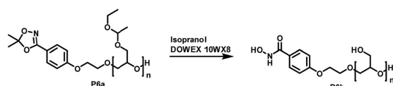
Scheme 6 Reaction scheme for cleavage of the protecting group in HAA-PEEGE releasing both the hydroxyl groups as well as the hydroxamic acid moiety.
