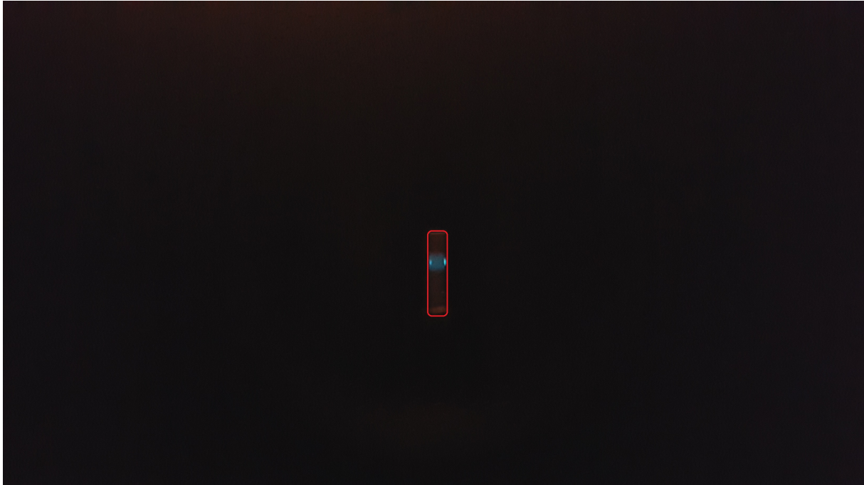
Figure 4.19: Photo taken from the position of the scat-PMT demonstrating its field of view, with the slit window (red) and the beam (teal). The beam is in good view and no reflection at the liquid surface is visible.
