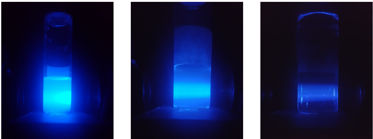
Figure 4.25: Colloid samples with various concentrations illuminated from the right. The leftmost picture shows the original sample with a concentration of c = 5.8 \cdot 10^{18} \text{ m}^{-3} and a Rayleigh scattering length of \Lambda_{\text{Ray}} = 5.02 \text{ mm} at 430 nm. The next two pictures show dilutions with water in ratios of 1:10 and 1:100, yielding ten and a hundred times longer scattering lengths, respectively. Note the visible drop in intensity in the leftmost sample with a scattering length smaller than the diameter of the glass vial.
