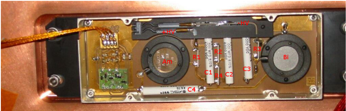
Figure 11.14: The standard configuration of the basic monitor as it is used in ATLAS detector (here just before complete construction) [240]. The red description of the components is based on the convention given in Figure 11.11.
