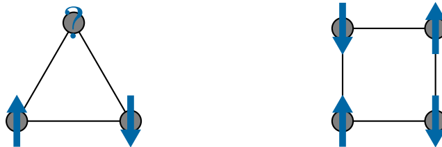
FIGURE 5.9: Antiferromagnetic interaction on the triangle leads to geometric frustration, because the spins can not satisfy the AF exchange interaction for all bonds simultaneously. Antiferromagnetic interaction on the square lattice, or any other bipartite lattice does not lead to frustration.
