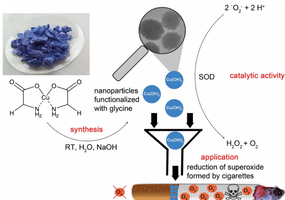
Fig. 1. Synthesis, enzymatic activity, and application of Gly-Cu(OH) 2 NPs. Cu(Gly) 2 was prepared by mixing aqueous solutions of copper(II) acetate and glycine. Addition of NaOH to a solution of Cu(Gly) 2 in water at room temperature (RT) led to the formation of Gly-Cu(OH) 2 NPs with high intrinsic SOD activity. As-synthesized NPs as part of cigarette filters reduce the concentration of superoxide radicals, produced by commercial cigarettes.
