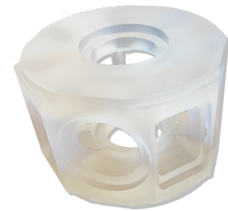
Fig. 4.6: Photo of the Zerodur MOT chamber body with 60 mm diameter and 40 mm height. Reprinted from reference [120].
