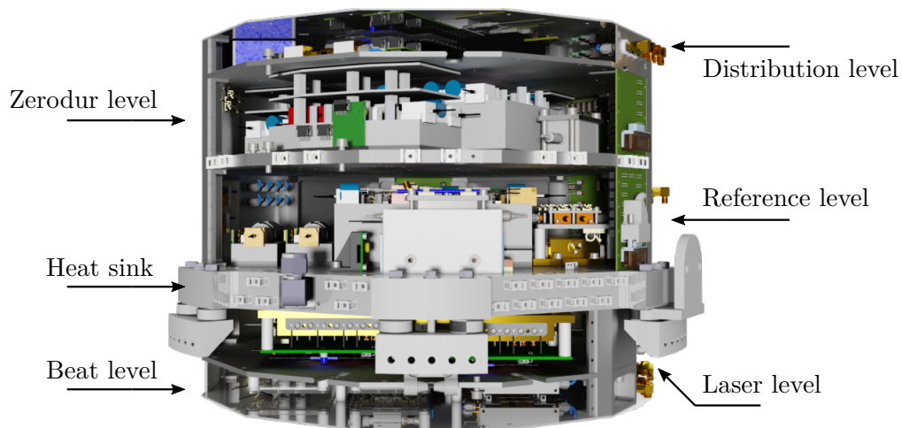
Figure 3.2: CAD rendering of the laser system for MAIUS-2/-3 with 458 mm diameter and 319 mm height (without mounting brackets). Adapted from reference [79].
