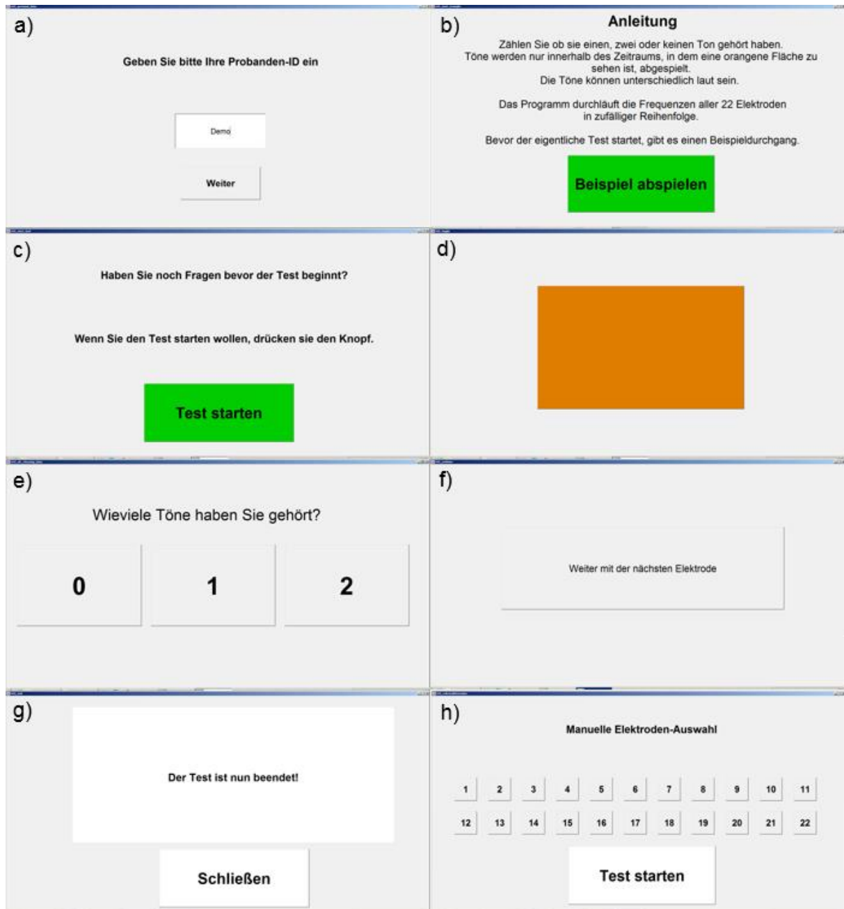
Figure 23. GUI screenshots: a) starting window, entering the patients' ID; b) instructions and button to play an example; c) window with a button to begin the application; d) orange box, which is only visible during the time stimuli can be perceived; e) response window; f) window, with 'continue with the next electrode' button, that is displayed after the three consecutive runs for one electrode are finished; g) finishing window at the end; h) window that is shown at the start if the option to manually select electrodes for testing was chosen.
