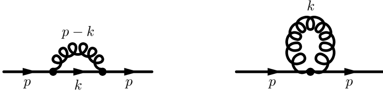
Figure 2.1: The 1-loop contribution to the fermionic self-energy consists of a sunset (left) and a tadpole (right) diagram.
