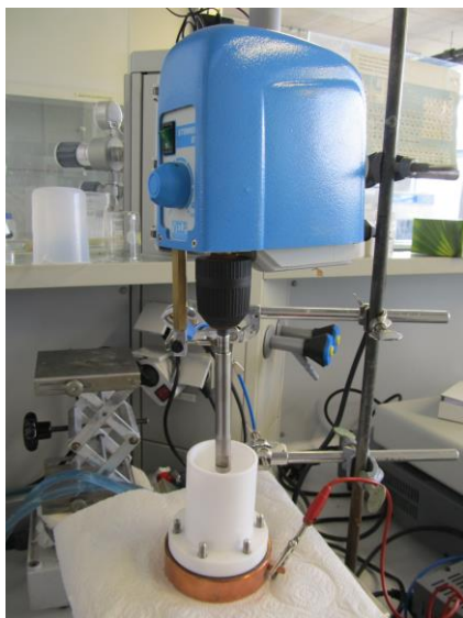
Figure 6.5: Photograph of the homemade rotating electrode showing the motor and the stirring part.
