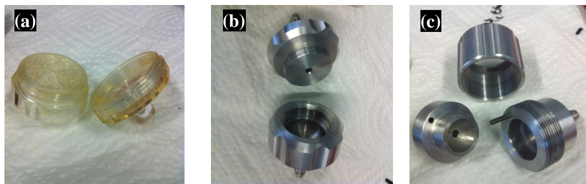
Figure 4.70: Photographs of tested filter holders: (a) Commercial 25 mm plastic filter holder (Whatman), (b) reproduction from aluminum for 16 mm discs, and (c) manufactured holder with device against twisting.
