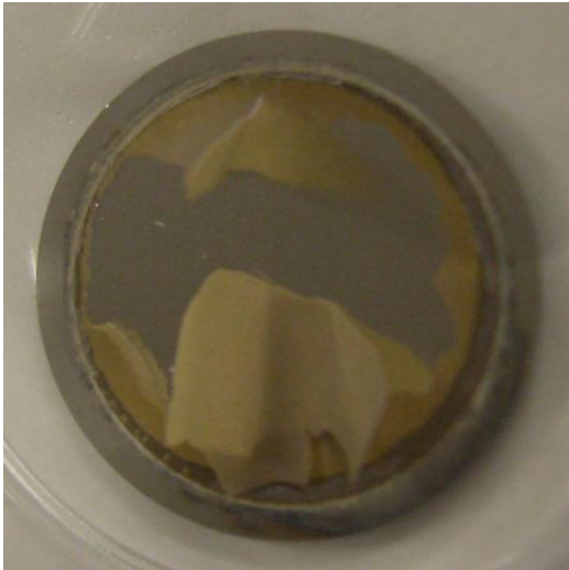
Figure 3.7: Photograph showing the curling of thick ATO layers from the underlying metal.
