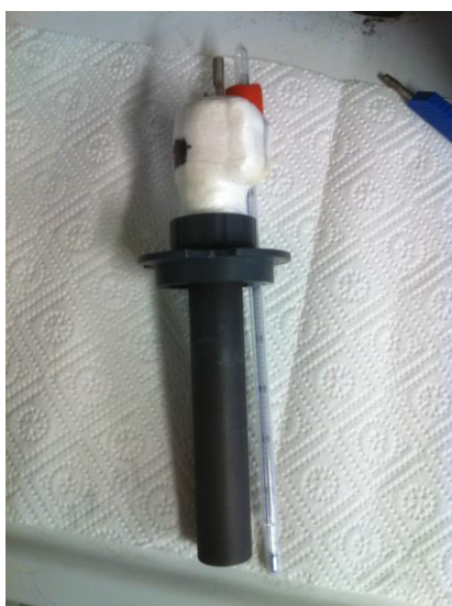
Figure 6.2: Photograph of a graphite rod electrode with Centering Device and thermometer.
