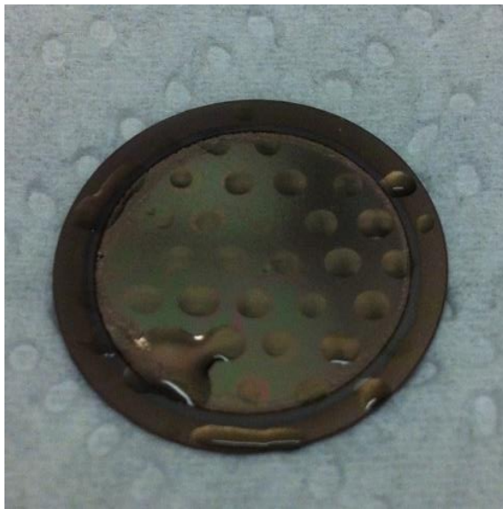
Figure 4.96: Photograph of a photolithographic pattern on a titanium surface, visualized by different wetting behavior.
