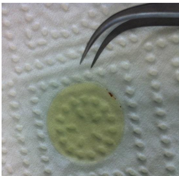
Figure 4.10: Photograph of an A2 16 mm oxide disc after the dissolution of supporting metal.
