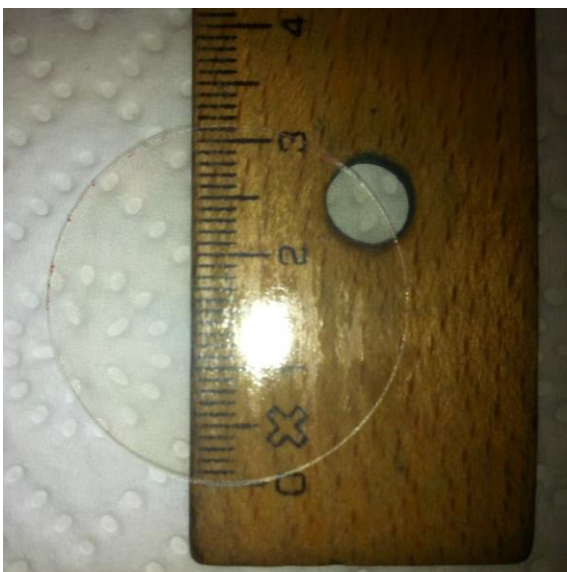
Figure 4.76: Photograph of an AAO membrane of 30 mm diameter (area of 7 \text{cm}^2 ).
