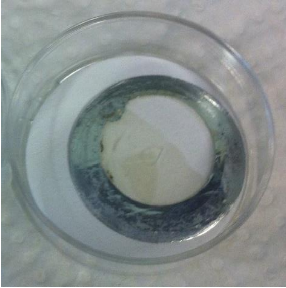
Figure 4.92: Photograph of a broken AAO window in its Al frame, produced by a modified DisA procedure.
