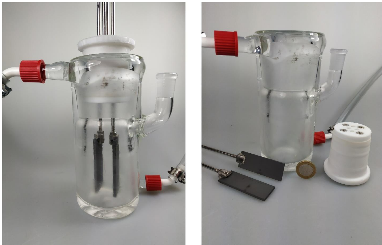
Figure 6: Beaker type-cell used for electrolysis of 50 mL electrolyte. The inner diameter is 4.69 cm. The outer shell is used in combination with a thermostat to control the temperature. Left: fully assembled cell, a condenser was added at the open end on the right. Right: parts of the setup with a 1 € coin for size comparison.
