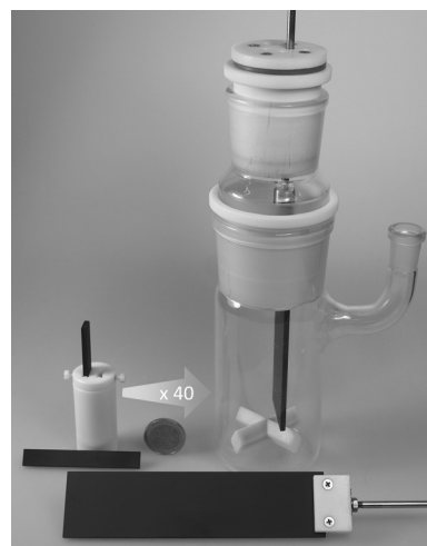
Figure 1. For the scale-up studies, 5 mL and 200 mL beaker-type cells were employed. For size comparison, a 2€ coin (diameter: 25.75 mm, ca. 1.01 inches) was placed between the two cells. See the Supporting Information for details.
