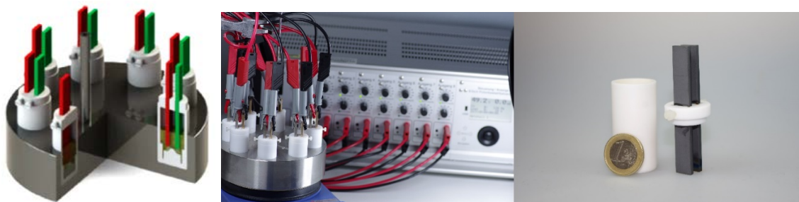
Fig. S1: Left: schematic 5 mL Teflon cells; Middle: The commercially available IKA Screenings System, IKA-Werke GmbH & Co. KG, Staufen, Germany; right: 5 mL Teflon cell with two parallel electrodes (size: 3 x 10 x 70 mm, 1 Euro coin for comparison, diameter: 23,25 mm).
