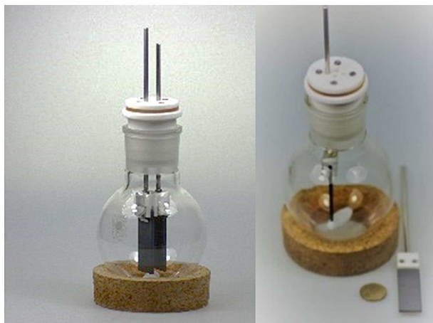
Figure 1. 500 mL round bottomed flask with Teflon plug and two BDD electrodes (14 cm × 3.5 cm × 0.3 cm) used in the scale up reaction. A 50 Eurocent coin for comparison. (diameter: 24,25 mm)
