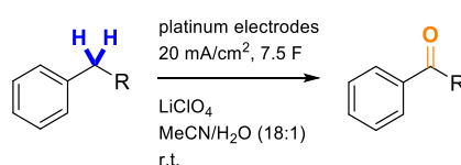
Scheme 4. Selective electrochemical benzylic oxidation towards ketones by Wang et al.
