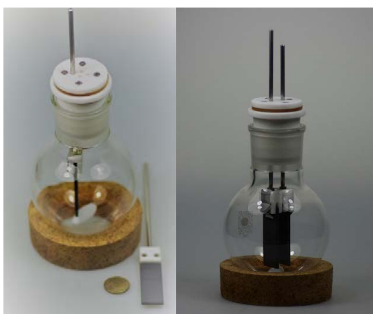
Fig. S2: 500 mL flask cell; left: BDD electrode removed; right: assembled. For size comparison one 50 Eurocent (diameter: 24,25 mm) coin is placed in front of the glass cell.
