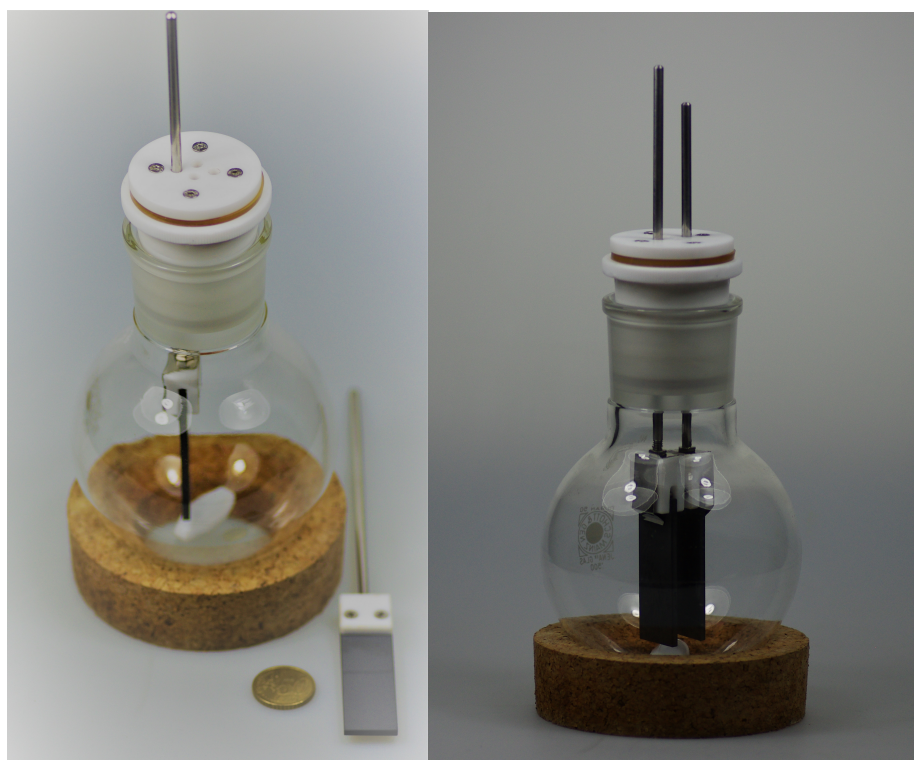
Fig. S2: 500 mL flask cell; left: BDD electrode removed; right: assembled. For size comparison one 50 Eurocent coin is placed in front of the glass cell.
