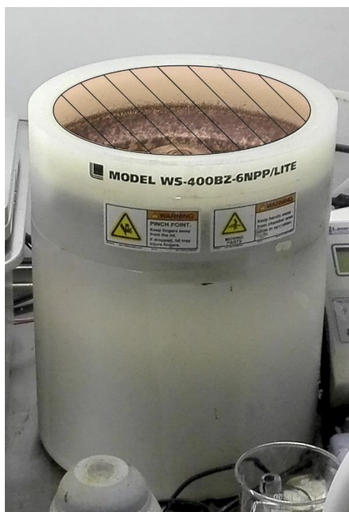
Figure 22: The indicated area is normally covered with a lid. Removal of that lid leads to improved gas exchange between spin-coater and glovebox.
