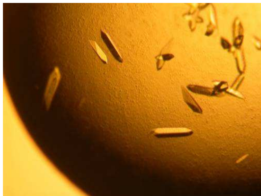
Figure 17. Crystals of native STR1. The rhombohedral crystals of STR1 belong to the space group of R 3 with unit cell parameters of a = b = 150.18 , c = 121.71 . The length of the crystals was approximately 0.08 - 0.2 mm. The complete data of STR1 in complex with strictosidine were collected to 3.0 Å resolution at the X13 beamline of EMBL Hamburg, Germany.
