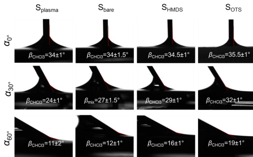
Figure 4.14. Meniscus angles of \text{CHCl}_3 ( \beta_{\text{CHCl}_3} ) at substrates with different surface energy for \alpha_0^\circ , \alpha_{30^\circ} and \alpha_{60^\circ} .
