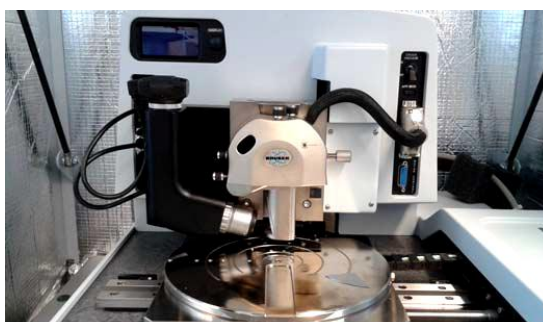
Figure 7.4. Dimension Icon FS atomic force microscope..
