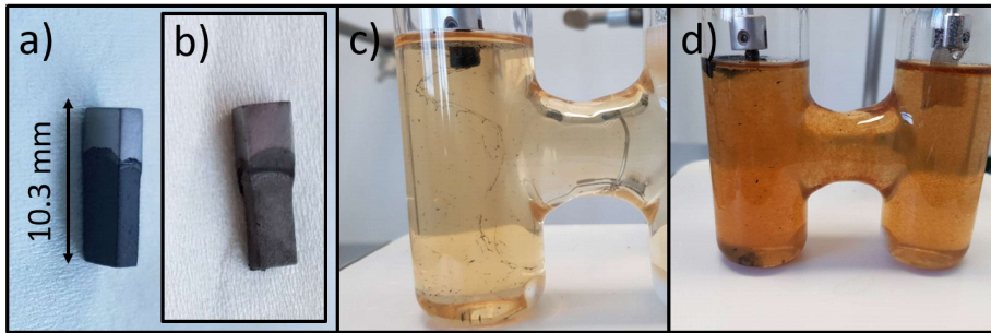
Figure S. 39: Electrolysis in saturated NaCl solution applying a pre-oxidized composite sample as anode upon varying potentials with U_{\max} = 10 V. Pre-oxidized anode before (a) and after (b) the electrolysis. Electrolysis cell at 6.5 V (c) and after applying 10 V (d).
