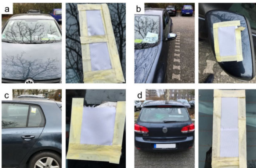
Figure S12. Photographs of the superomniphobic fabrics on the car after 257 days of outdoor exposure. a) Superomniphobic fabrics fixed on the front window. b) Fabric fixed on the left mirror. c) Fabric fixed at the rear side windows. d) Fabrics fixed at the back window. All superomniphobic fabrics remained white without any obvious stains.
