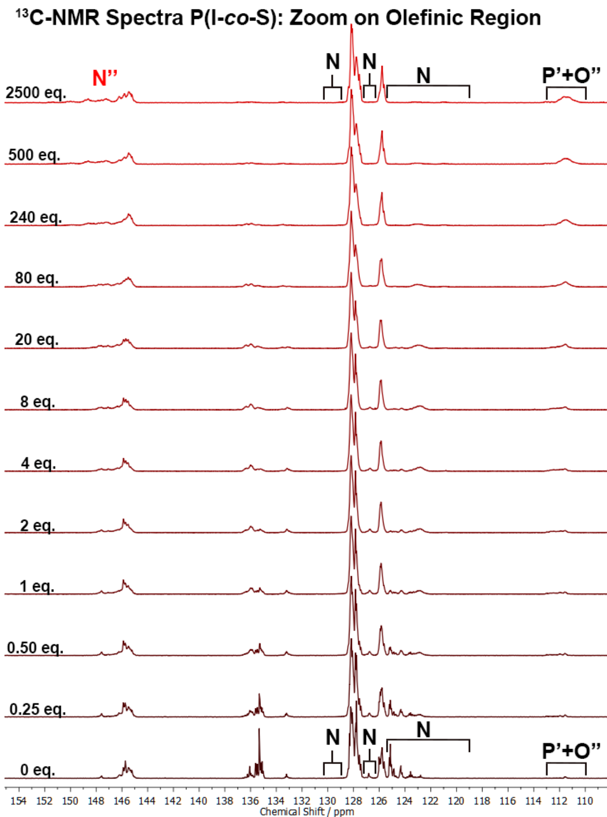
FIGURE S20F Zoom of the olefinic and aromatic region: Stacked Inverse Gated ^{13}\text{C} NMR spectra (150 MHz, \text{CDCl}_3 ) of the 50% _{\text{mol}} P(I-co-S) copolymers. The equivalents of THF in respect to the active chain ends, was increased as indicated at the spectra. Black font: separated signals used for data evaluation, red font: overlaid signals.
