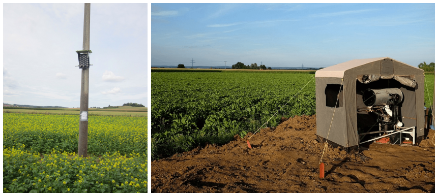
Figure 5.8: Measurement set-up of the LP-DOAS at the barn station. Left: the reflector amidst crop fields. Right: the telescope next to the barn.
