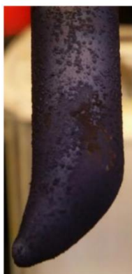
Figure 1. Photograph of Au(TPP) sublimed onto the cold finger of the sublimation apparatus.
