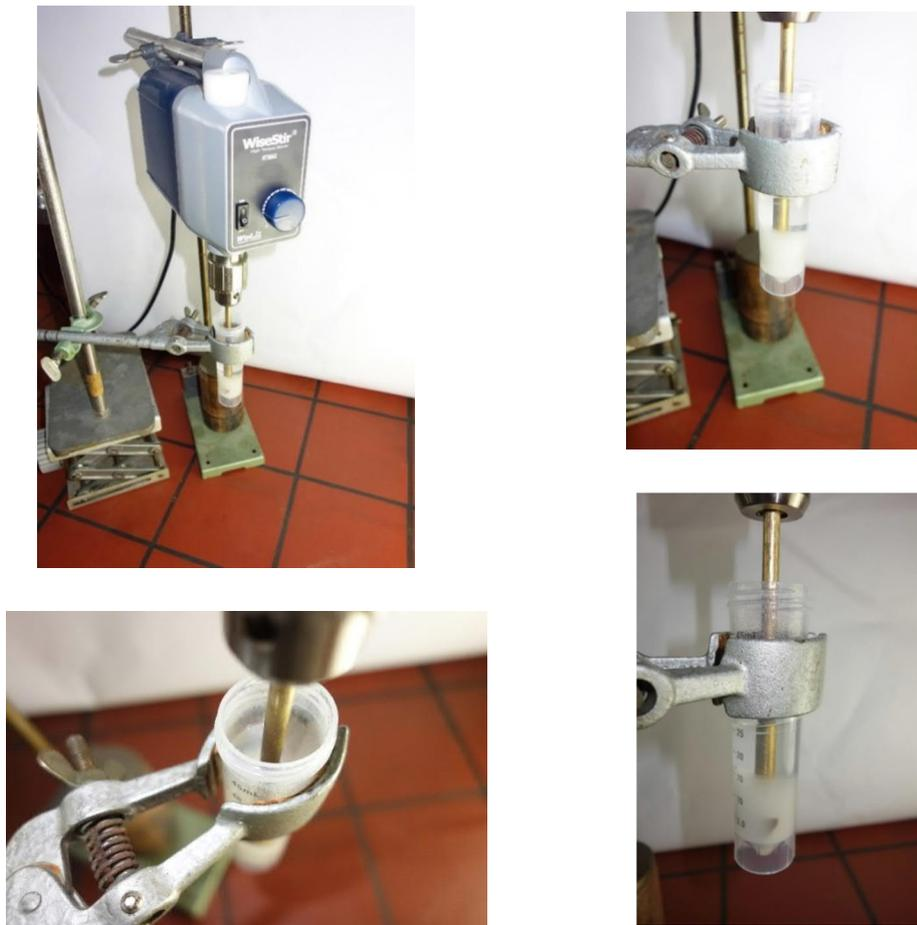
**Figure 15:** Vane spindle mixing device.
