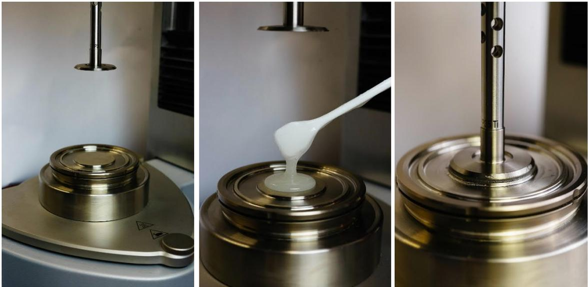
**Figure 17:** Measurement setup using a parallel-plate geometry
