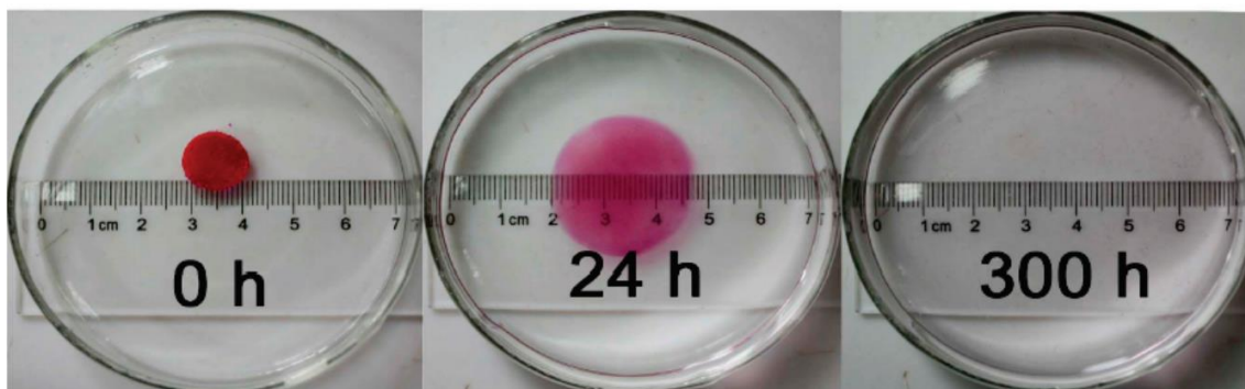
Figure 14: Swelling and degradation of PEG-PPE-hydrogels loaded with Nile red. (Reprinted with permission from reference 190 . Copyright 2011 American Chemical Society.)
