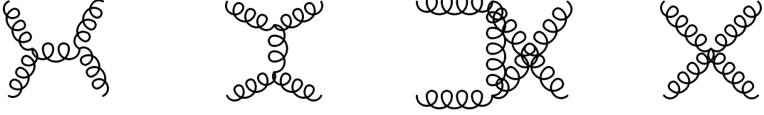
Figure 2.12: Diagrams for 2 \rightarrow 2 processes involving two gluons in the initial and final state. From left to right: s -channel, t -channel, u -channel and quartic vertex.
