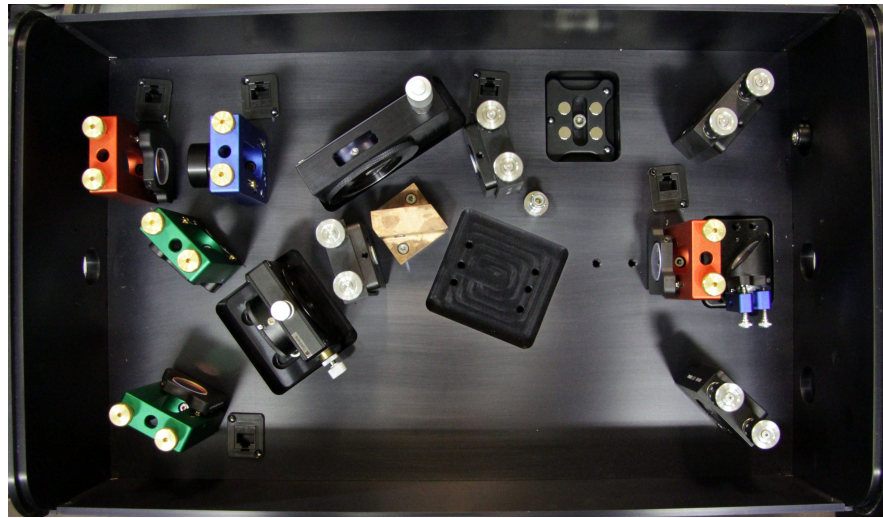
Figure 5.3: Photograph of a CERN-Ti:Sa cavity. The mirror mounts are color-coded to reduce the likelihood of accidental mis-tuning. Green mounts control the pump beam. The red mounts hold the high reflecting and the output coupling cavity mirror. The blue mount holds an etalon for manual control. In this cavity, no Pockels cell is installed, but its square mounting slot can be seen on the baseplate.
