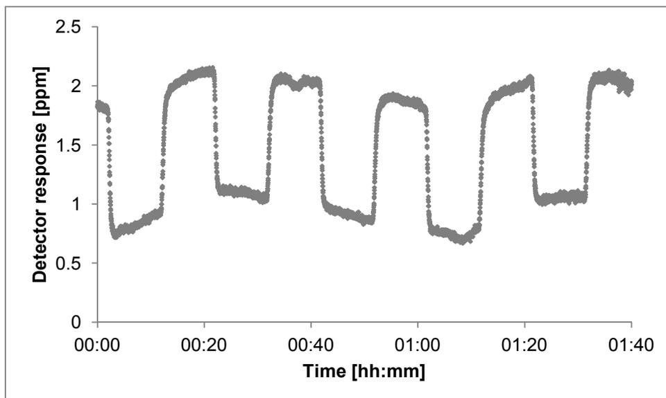
Figure 20: CO<sub>2</sub> signal arriving at the IRGA when continuously flushing the oxidation unit with helium. The oxygen addition is switched on and off every ten minutes.
