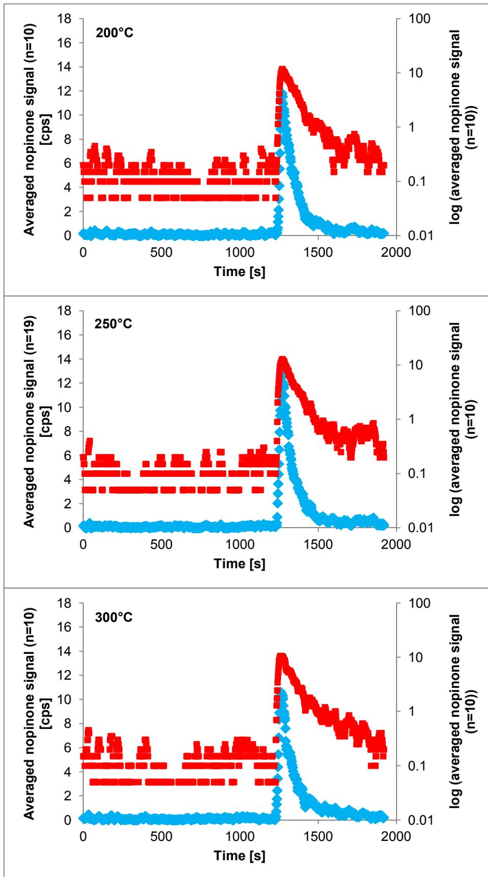
Figure 37: Single nopinone desorption courses (primary y-axis: blue diamonds) for different temperatures (200°C, 250°C, 300°C) shown together with the respective desorption peaks as logarithmic plots (secondary y-axis: red squares) for a more detailed view of the desorption course.
