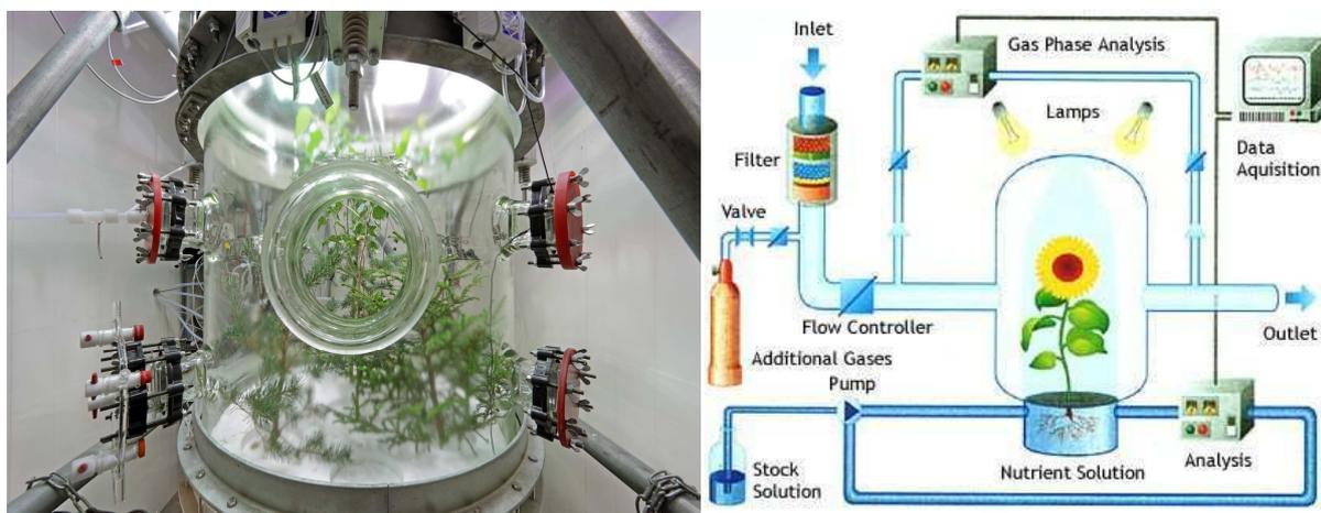
Figure 15: Setup of the Jülich Plant Atmosphere Chamber (JPAC).<sup>10</sup>
