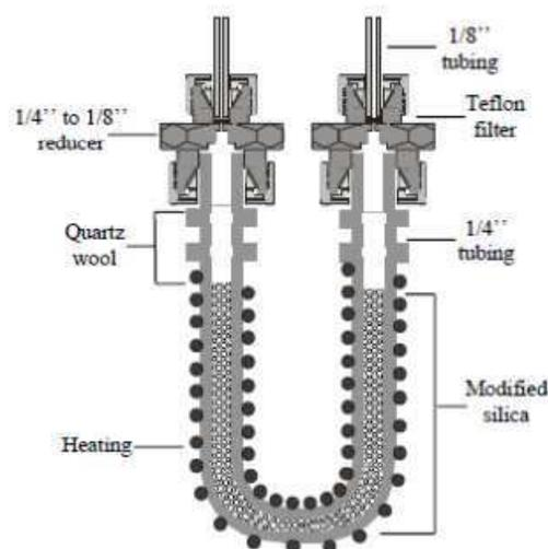
Figure 9: Schematic illustration of the CO<sub>2</sub> preconcentration unit. Support frame, ventilator and thermocouple are not shown (Dindorf 2006).
