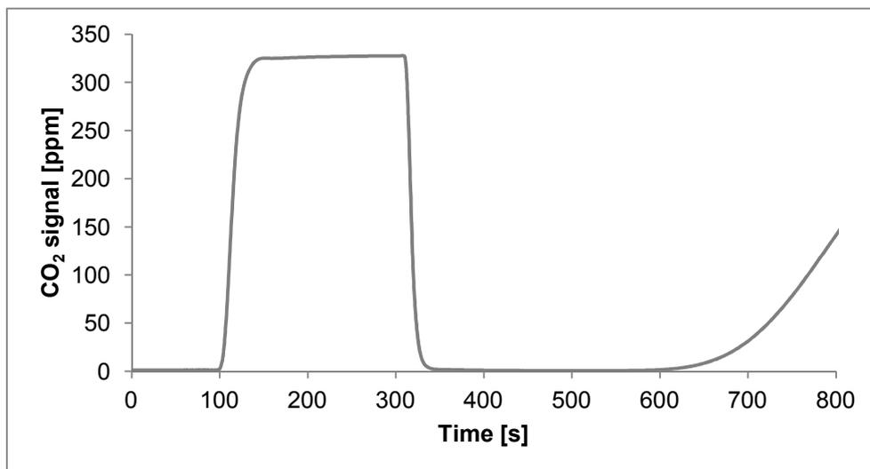
Figure 16: Course of the breakthrough volume determination. The first 60 s show the zero signal from helium bypassing the CO<sub>2</sub> preconcentration unit. After 60 s it is manually switched to the CO<sub>2</sub> standard gas which is still bypassing the unit. After 3 min the preconcentration unit is switched into the CO<sub>2</sub> in synthetic air gas stream by the electrical 3-way-2-position valves. The uptake of the CO<sub>2</sub> can be identified by the decrease of the signal to zero.
