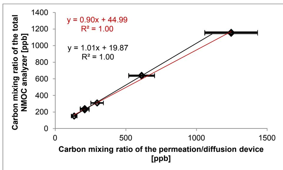
Figure 39: Correlation between the carbon mixing ratio values from isoprene obtained with the total NMOC analyzer (y-axis) and the calculated values from the permeation/diffusion devices (x-axis) (with an uncertainty of  $\pm 15\%$ ). The red line shows the linear regression including all isoprene mixing ratios. The black fit does not include the highest mixing ratio.
