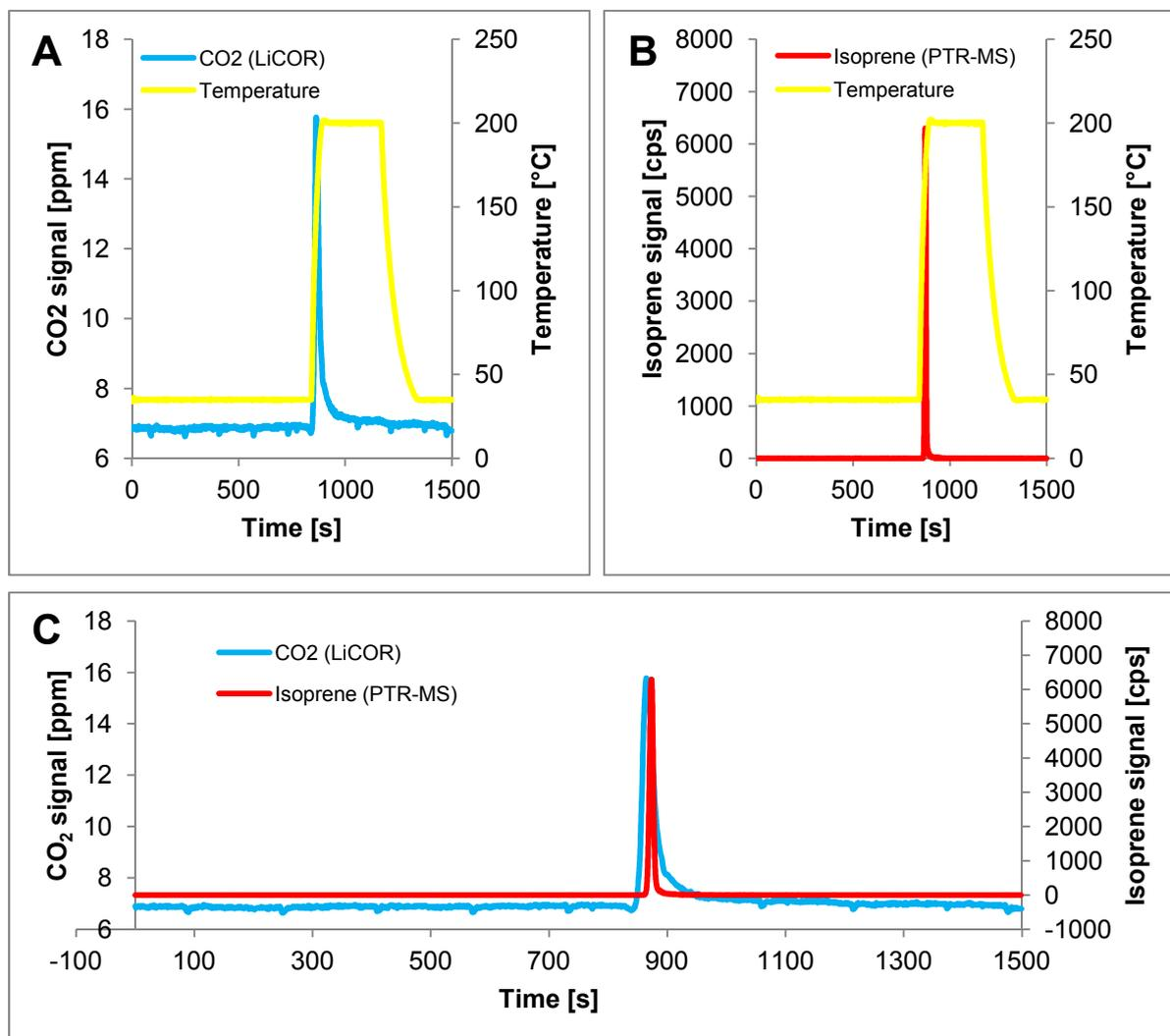
Figure 34: A: Desorption course of sampled CO<sub>2</sub> (blue line) from the NMOC solid adsorbent unit and the corresponding temperature course (yellow line). B: Course of the isoprene signal (red line) during desorption with the temperature course. C: CO<sub>2</sub> signal (primary y-axis) together with the isoprene signal (secondary y-axis).
