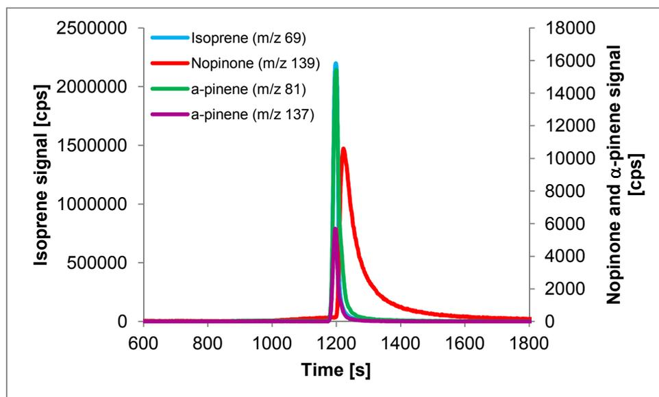
Figure 38: Compound signals after thermal desorption. As the signal intensity was different for the chosen compounds the isoprene signal was plotted on the primary y-axis and the other compounds (nopinone and  $\alpha$ -pinene) on the secondary y-axis.
