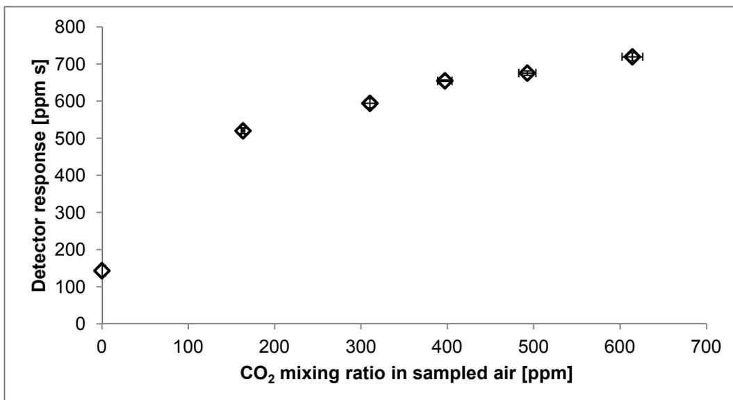
Figure 26: Detector response of repeated zero air measurements containing different CO<sub>2</sub> mixing ratios. The black diamonds represent the mean average ( $n > 3$ ) of the measured values from the total NMOC analyzer with the corresponding average CO<sub>2</sub> mixing ratios including standard deviation.
