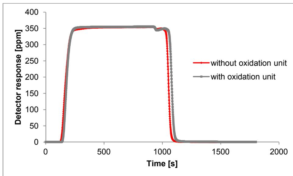
Figure 24: CO<sub>2</sub> uptake and release test with the Pt-Rd wire catalyst. The red line represents the CO<sub>2</sub> signal of the standard gas flushed through the system without the oxidation unit and the grey line including the oxidation unit.
