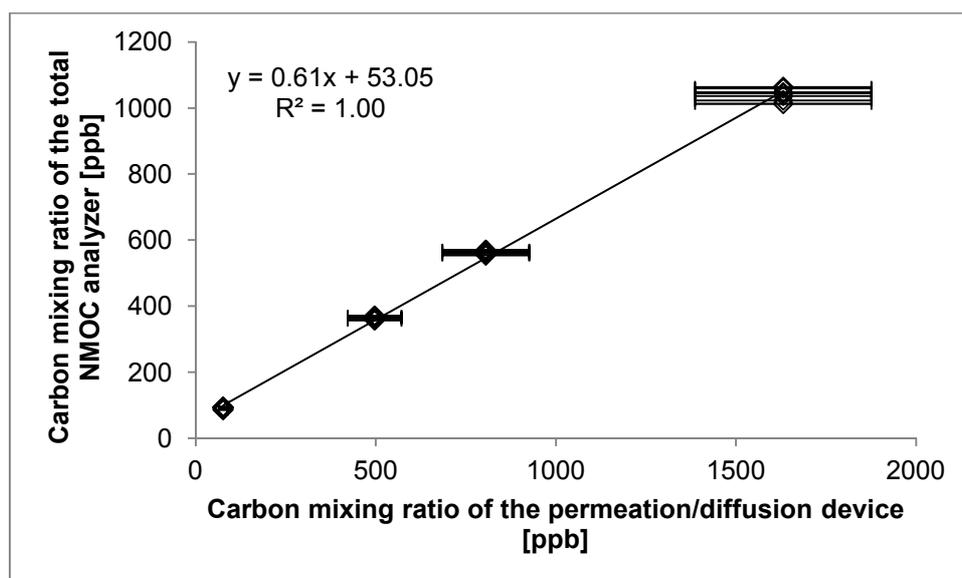
Figure 40: Correlation between the carbon mixing ratios from  $\alpha$ -pinene obtained with the total NMOC analyzer (y-axis) and the calculated values ( $\pm 15\%$ ) from the permeation/diffusion devices (x-axis).
