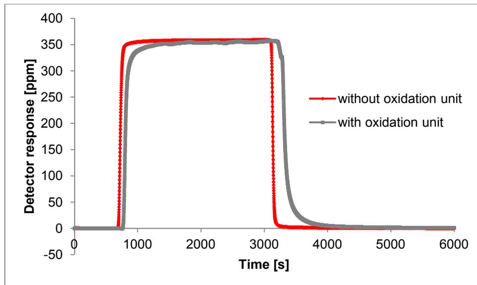
Figure 21: CO<sub>2</sub> uptake und release test with the Pt catalyst material. The red line represents the CO<sub>2</sub> signal of the standard gas flushed through the system without the oxidation unit and the grey line including the oxidation unit.
