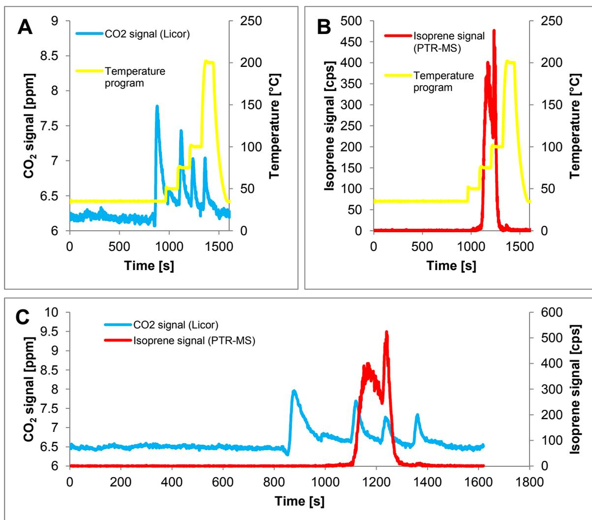
Figure 35: A: CO<sub>2</sub> signal after desorption in relation to the temperature. B: Isoprene signal in relation to the temperature. C: Comparison of the CO<sub>2</sub> and the isoprene signal (primary y-axis: CO<sub>2</sub> signal; secondary y-axis: isoprene signal).
