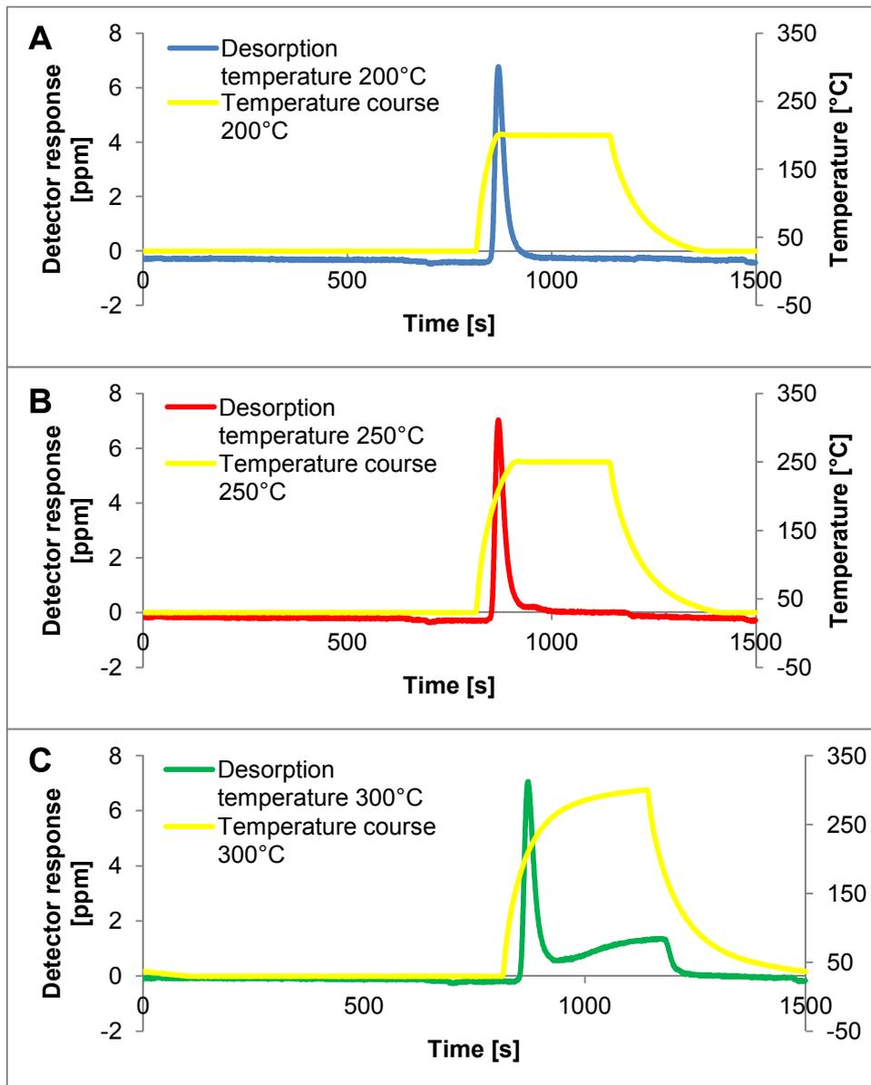
Figure 32: CO<sub>2</sub> background signals (primary y-axis) from an ambient zero air measurement with different desorption temperatures (A = 200°C, B = 250°C, C = 300°C). The colours are corresponding to Figure 31. Yellow represents the temperature course of the measurement run (secondary y-axis).
