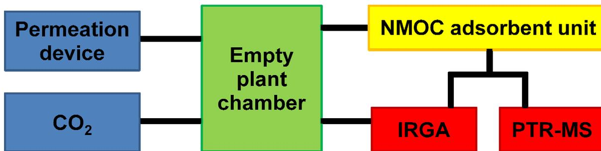
Figure 33: Schematic setup for the compound measurements with the NMOC solid adsorbent unit.
