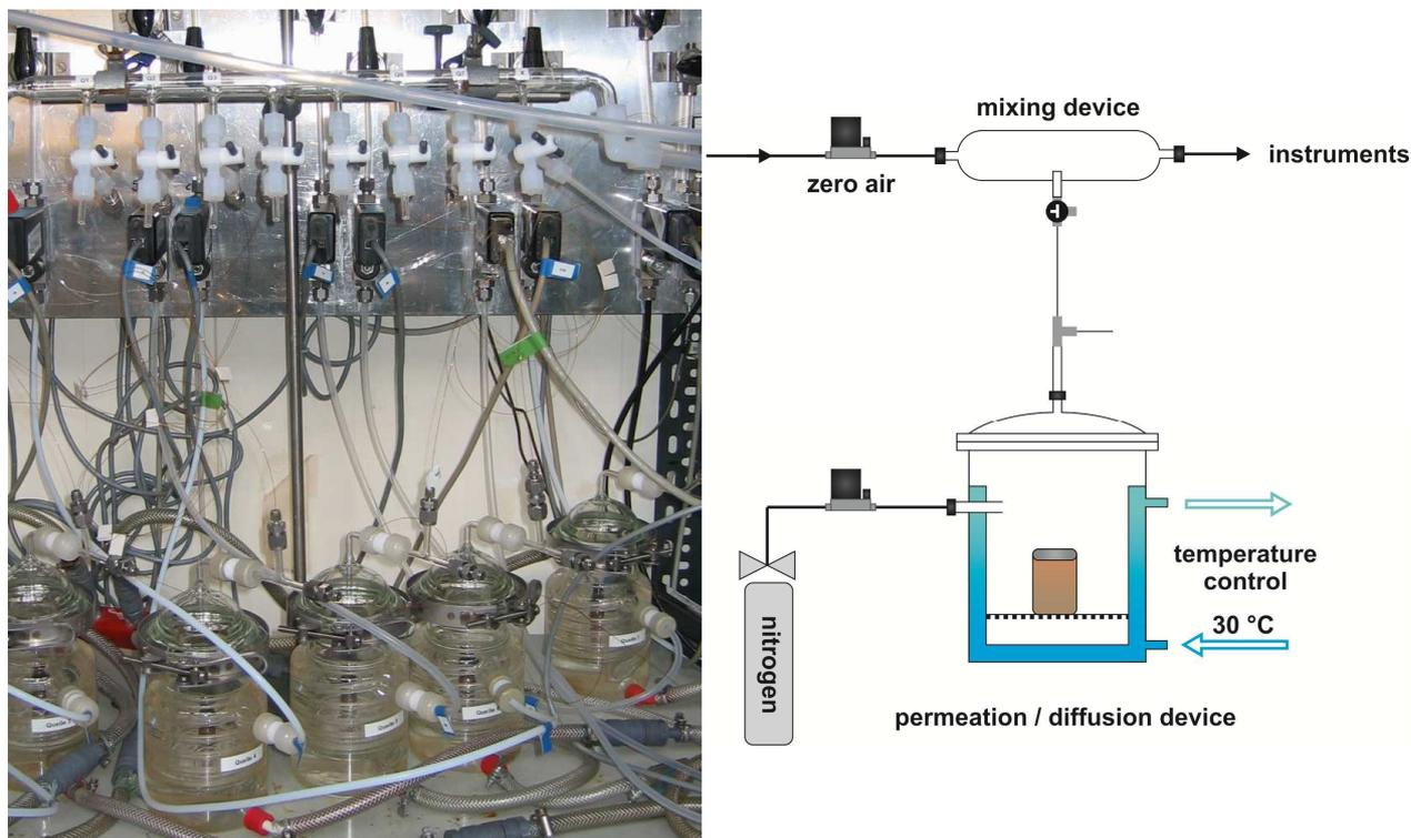
Figure 14: Setup of the permeation/diffusion devices.
