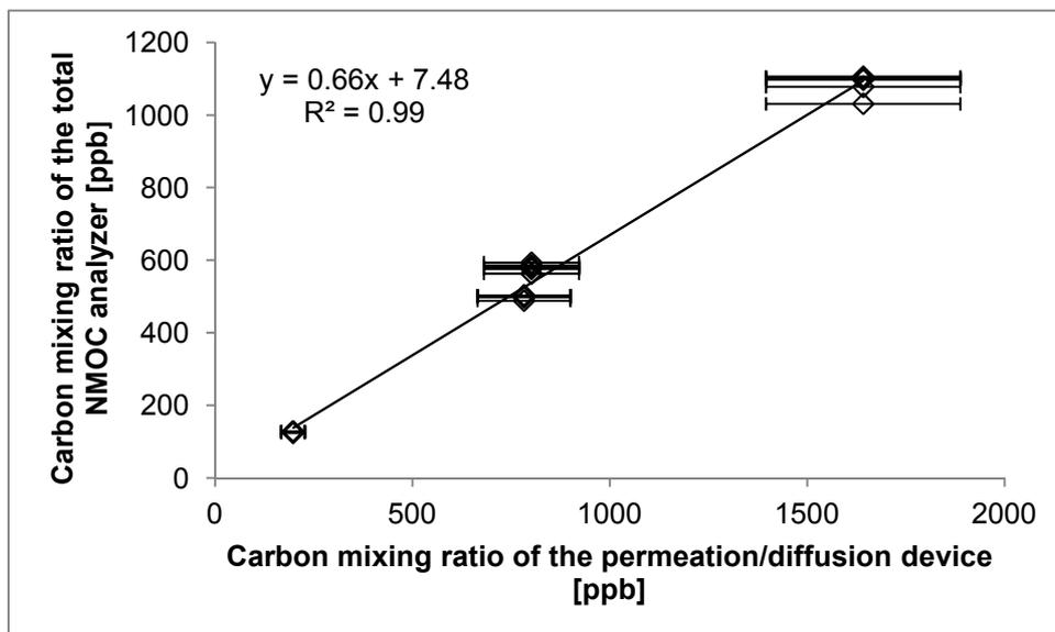
Figure 41: Correlation between the carbon mixing ratios from nopinone obtained with the total NMOC analyzer (y-axis) and the calculated value from the permeation/diffusion devices (x-axis) (with an uncertainty of  $\pm 15\%$ ).
