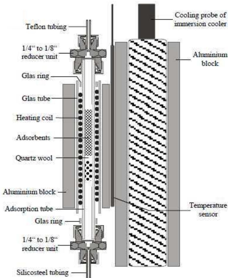
Figure 11: Schematic setup of the NMOC solid adsorbent unit (Dindorf 2006).
