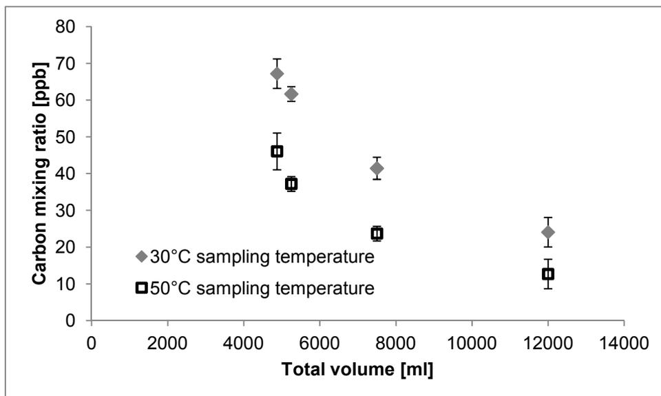
Figure 30: Decrease of the carbon signal ( $n > 3$  including standard deviation) with increase of the flush volume considering the total volume (sample volume = 3000 ml plus flush volume).
