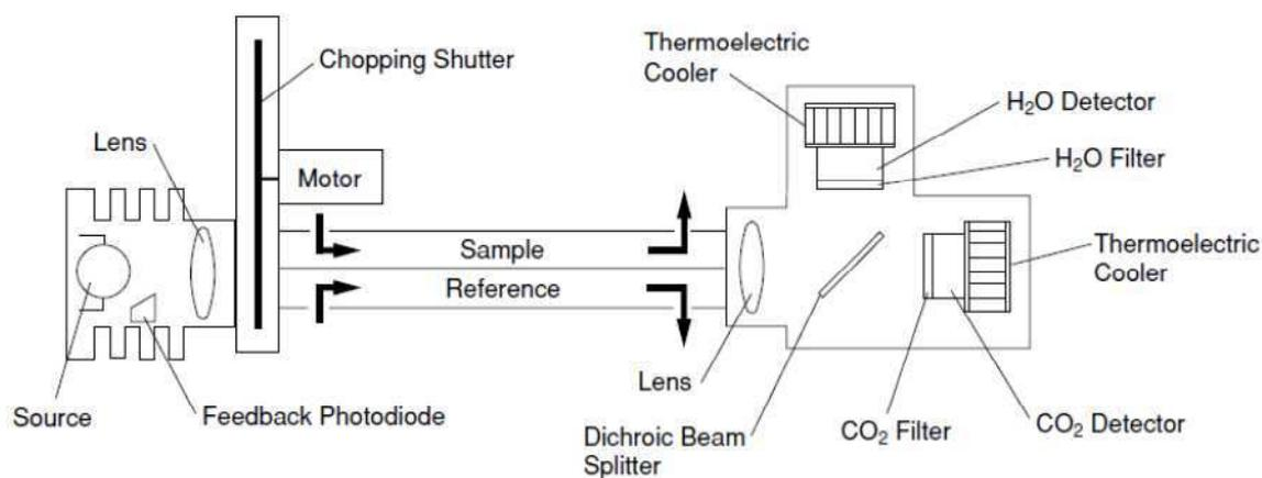
Figure 8: Schematic setup of the infrared gas analyzer.<sup>8</sup>
