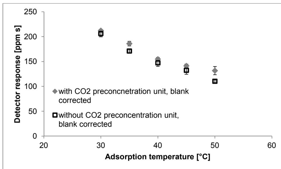
Figure 28: Decrease of the CO<sub>2</sub> background signal ( $n > 3$  including standard deviation) with increasing sampling temperature. The black squares represent the values obtained without the CO<sub>2</sub> preconcentration step and the grey diamonds show the results for the measurement including the CO<sub>2</sub> preconcentration unit. Both results are blank corrected.
