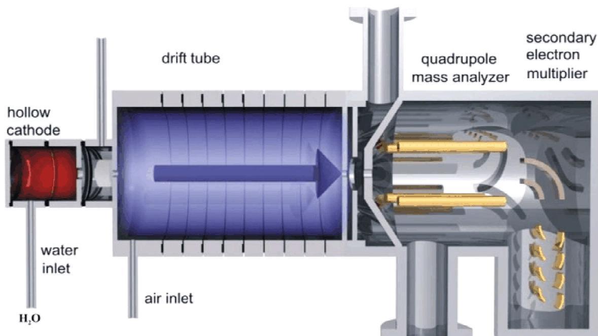
Figure 13: Schematic setup of the PTR-MS.<sup>9</sup>
