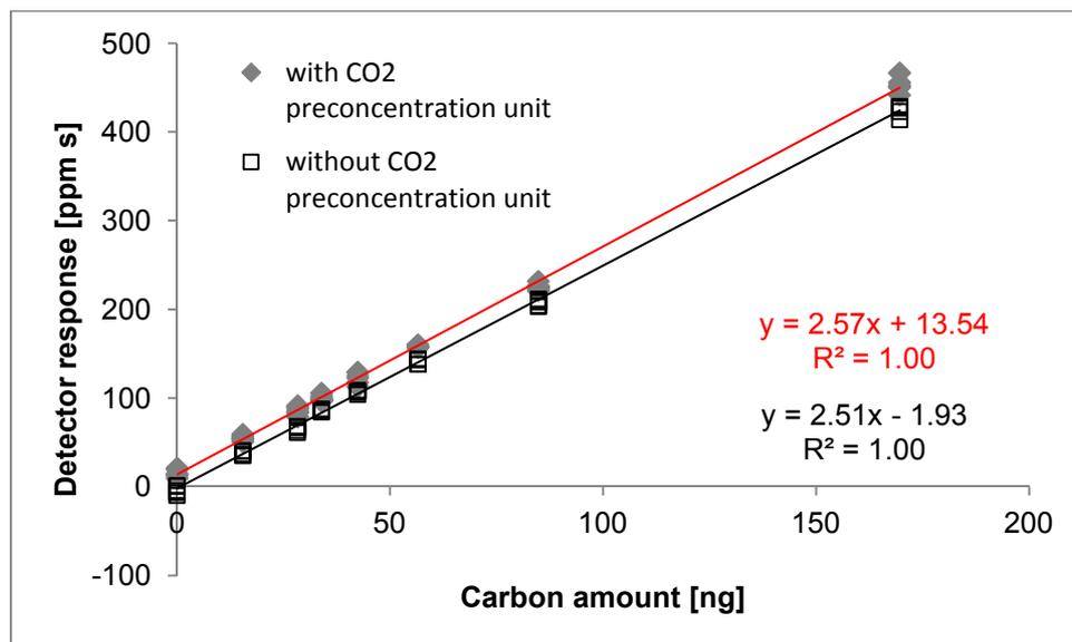
Figure 17: Signal development of different CO<sub>2</sub> ratios (CO<sub>2</sub> standard gas diluted in different volumes of helium (6.0) (see Table 4) including the CO<sub>2</sub> preconcentration unit (grey diamonds and red linear regression line) and without the CO<sub>2</sub> preconcentration unit (empty squares and black linear regression line). A shift to to higher values was observed when using the unit.
