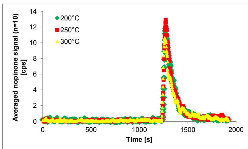
Figure 36: Signal development for nopinone desorbed at different temperatures (200°C, 250°C, 300°C). Each nopinone value was averaged over 10 individual values (n=10).
