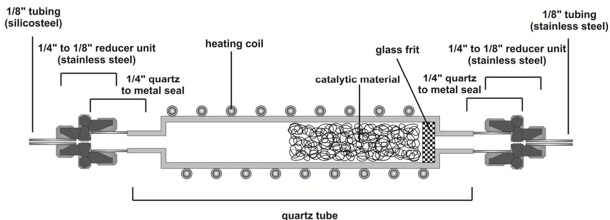
Figure 10: Schematic figure of the new oxidation unit. Thermocouple, power supply and insulation material are not shown.
