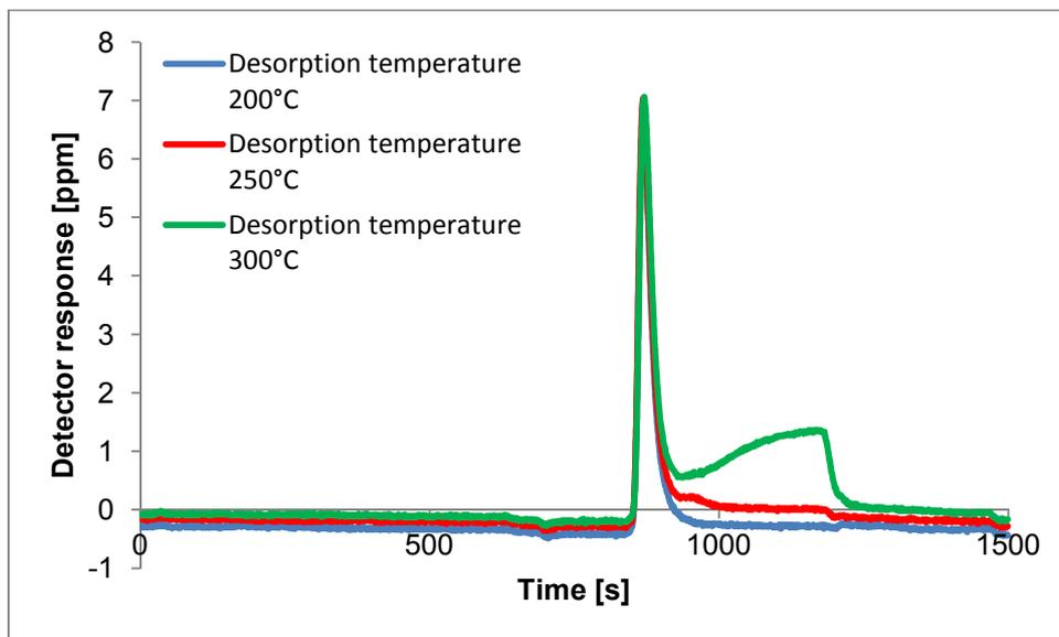
Figure 31: Different CO<sub>2</sub> background signals from zero air sampling containing CO<sub>2</sub> in ambient mixing ratios. The blue line shows the course with a desorption temperature of 200°C, the red one the CO<sub>2</sub> signal for the run with a desorption temperature of 250°C and the green line shows the result for 300°C desorption temperature.
