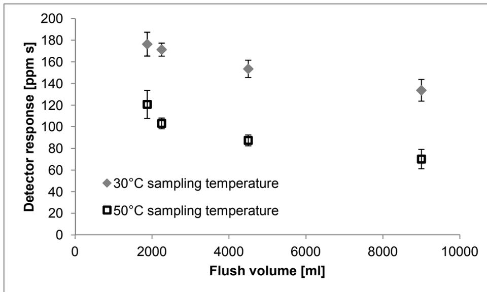
Figure 29: Decreasing CO<sub>2</sub> blank values with increasing flush volume. The grey diamonds represent the average values ( $n > 3$  including standard deviation) of a flush volume experiment with a sampling temperature of 30°C. The black squares are the mean results ( $n > 3$  including standard deviation) with a sampling temperature of 50°C. Both measurements were carried out excluding the oxidation unit and the CO<sub>2</sub> preconcentration unit. All mean values are blank corrected.
