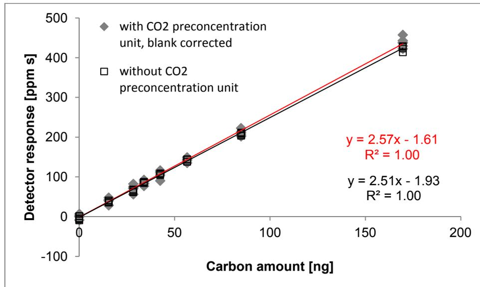
Figure 18: Comparison between the blank corrected values of measurements including the CO<sub>2</sub> preconcentration unit (grey diamonds) and the values without the CO<sub>2</sub> preconcentration unit (empty squares) of different CO<sub>2</sub> ratio measurements.
