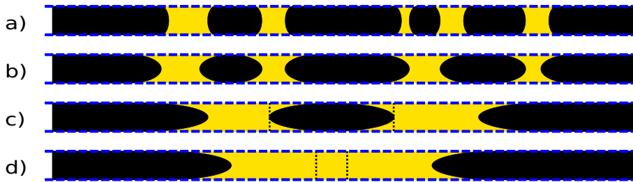
Figure 8.8.: Schematic representation of the different processes influencing the particle distribution perpendicular to the walls in a narrow quasi two-dimensional system. (a) Particles rapidly form groups of the size of wall separation and connect to the walls. (b) The strong depletion force acting at the colloids (yellow areas) leads to a further flow of this species to the walls. (c) Domains combine but the colloids still move into the direction of the walls. (d) Saturation of the colloidal drift towards the walls and further connection of domains redistributing colloid layers close to the walls among the center region (indicated by the yellow area enclosed by vertical dotted lines).
