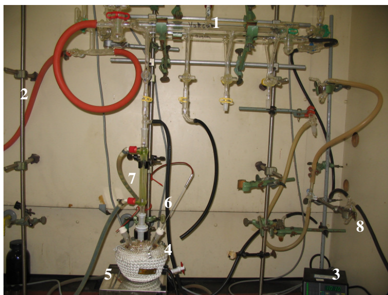
Figure 3.1: Experimental set up for QD synthesis: 1. schlenk glass ware; 2. to vacuum pump; 3. pressure indicator; 4. heating mantle; 5. magnetic stirrer; 6. thermocouple; 7. condenser; 8. to argon gas cylinder.
